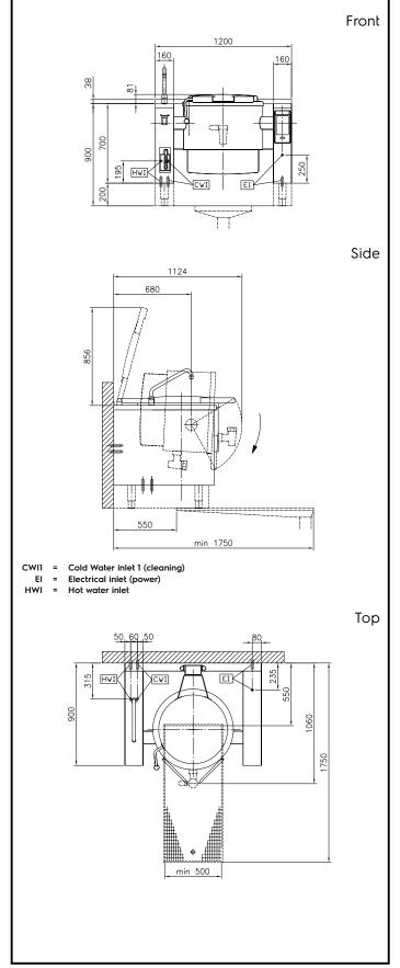
ProThermetic Sprint Electric Tilting Boiling Pan, 100lt Hygienic Profile, Freestanding
